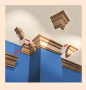
**Finishing:** To obtain a nice finish, fill the nail holes and the joints with a latex caulking. If you wish to paint your mouldings, lightly sand the surface with a fine sandpaper, apply a coat of primer and then one or two coats of your favourite paint. If the mouldings are pre-painted, you can touch them up to correct imperfections.
